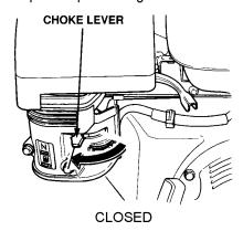
Figure 12. Choke Lever (Closed)
